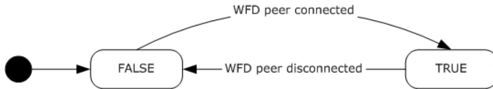
Figure 6: ObOb Connector WfdPeerConnected transitions
