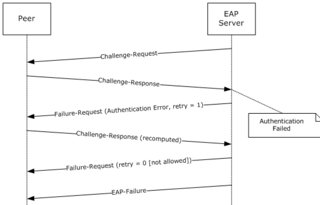
**Figure 6: Authentication failure with retry that also fails**
