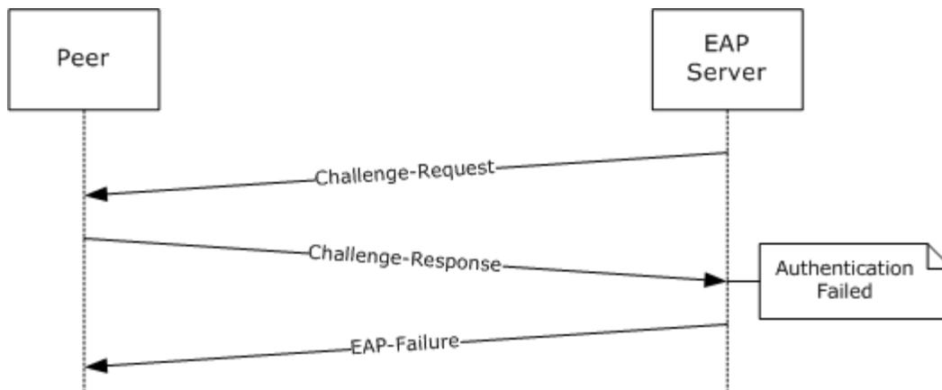
**Figure 7: Authentication failure with no retry allowed**
